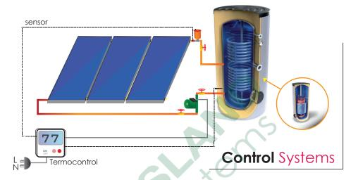
The system separates the collector and the heat storage tank. The tank can be arbitrarily placed, hot water storage tank repacement heating device. Collectors absorb solar energy light into heat water or heating medium circulated between the collector and the heat exchanger means to promote heat transfer between the collector and the natural flow of media devices, media devices through the heat exchange, thermal heat storage tank in the water.
